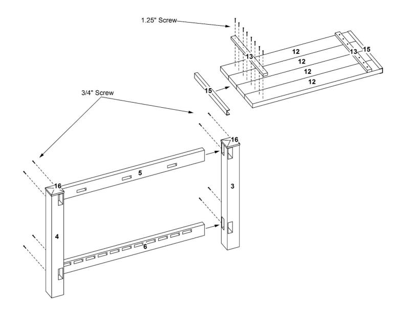
Insert one 51½" table rail (part 5) into 38" front right post (part 4). Insert one 51½" shelf rail (part 6) into 38" front right post. Insert free ends of table and shelf rail into 38" back left post (part 3). Using four ¾" screws per post, screw together potting bench front panel. Be sure all parts are fully inserted into posts before securing. Using included super glue tube, glue 4" sq. flat post cap (part 16) onto top of each post.
