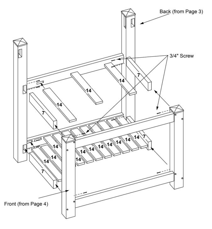
Insert four 22" side rails (part 7) into posts of potting bench pack panel (from page 3). Insert three 24½" table/shelf rails into table rail of back panel. Insert eleven table/shelf rails into shelf rail of back panel. Insert free ends of side rails and table/shelf rails into corresponding holes of potting bench front panel (from page 4). Using four ¾" screws per post, fasten together potting bench. Be sure all parts are fully inserted before securing.
