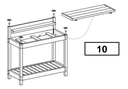
Apply PVC glue to inner edges of four 2" sq. post caps and place on top of each post. Set table top assembly into working area of potting bench. The table top is designed to be removed for easy and quick cleaning.
