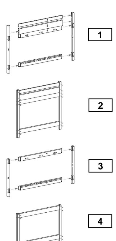
Insert  $\frac{7}{8}$ " x 3" x 46 $\frac{1}{2}$ " back rail (part 8) into top hole in back right post (part 2). Insert 1 $\frac{1}{2}$ " x 5 $\frac{1}{2}$ " x 46 $\frac{1}{2}$ " back rail (part 9) into top of large hole of back right post. Insert one table support (part 4), into bottom of large hole of back right post. Insert one shelf support (part 5) into bottom hole of right back post. Insert free ends of all rails into corresponding holes of back left post (part 1).
