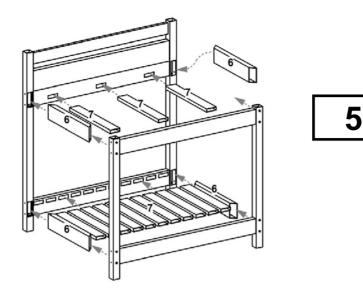
Insert three  $\frac{7}{8}$ " x 3" x 20¼" table/shelf rails (part 7) into table support of back panel. Insert eleven  $\frac{7}{8}$ " x 3" x 20¼" table/shelf rails (part 7) into shelf support of back panel. Insert two 1½" x 4" x 20¼" side rails (part 6) into back right and back left post. Insert free ends of all rails into corresponding holes of front panel.
