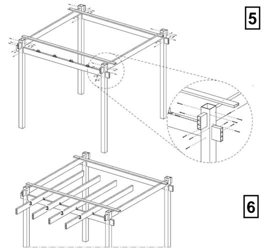
Using 2" painted screws, screw together all posts and supports.
