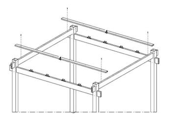
Lay two cross rail (part 4) onto upper supports. To set width of pergola, line up outer most holes of top rails with outer most pilot holes of upper supports. Using 1¼" painted screws, fasten top rails to upper support.
