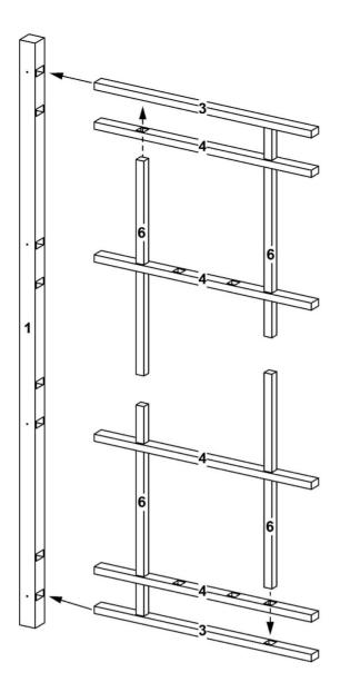
Starting at bottom of 74" left post (part 1), insert one 27½" outer cross rail (part 3) and two 27½" inner cross rails (part 4). When inserting two inner cross rails insert sides with four routed holes facing each other. Insert two 26½" vertical rails (part 6) through outer holes of inner cross rails and into outer holes of outer cross rail.
