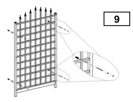
To secure to wall, slide 6" screw through clear screw backer. Insert screw through pre-drilled hole in post. To set trellis away from wall, slide screw through spacer tube. After securing, snap screw cap over the screw backer.
