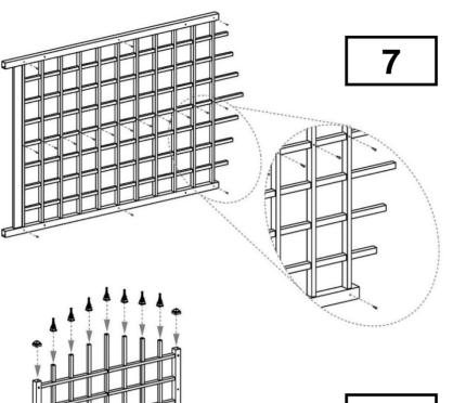
Using ¾" painted screws, screw together trellis. Be sure that all parts are fully inserted into posts before securing.
