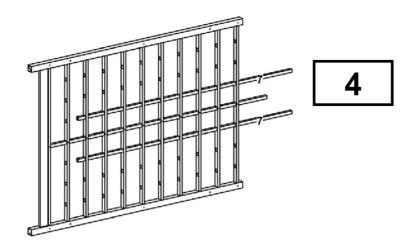
Working outward away from center, insert 82" vertical rails (part 7) through cross rails.
